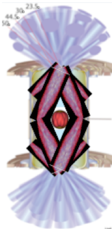
Figure 11: A NIF ignition target. Ninety-six NIF beams enter the target through both the top and bottom laser entrance holes. The hohlraum is composed of a high-Z cylinder filled with helium gas and contains a capsule of DT in the center.
